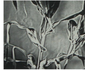
Airflow around the leaves of a corn plant is visualized using schlieren imager for agronomical research.
